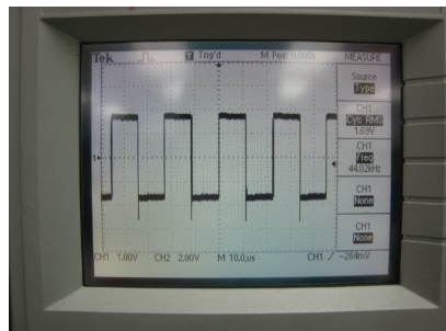
U1001 Pin 12 - Left/Right clock (PCM), 44.1kHz
